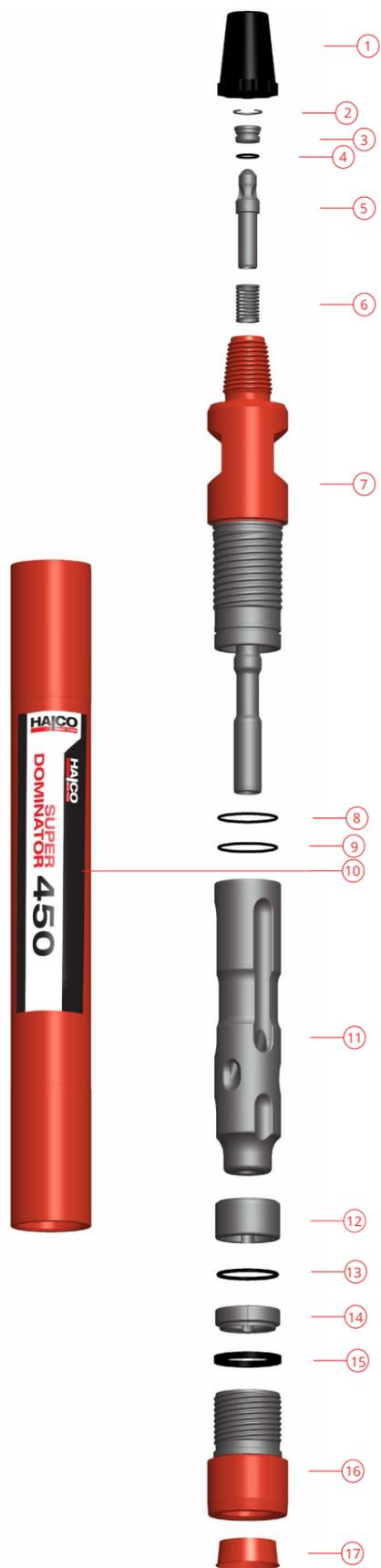
**A.** Before assembly ensure that all components are cleaned, greased and lubricated. Lay out components in the order of the illustration above for ease of identification.
