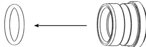
**E.** Remove the Chuck Lock Ring (15) from the Chuck (16).
